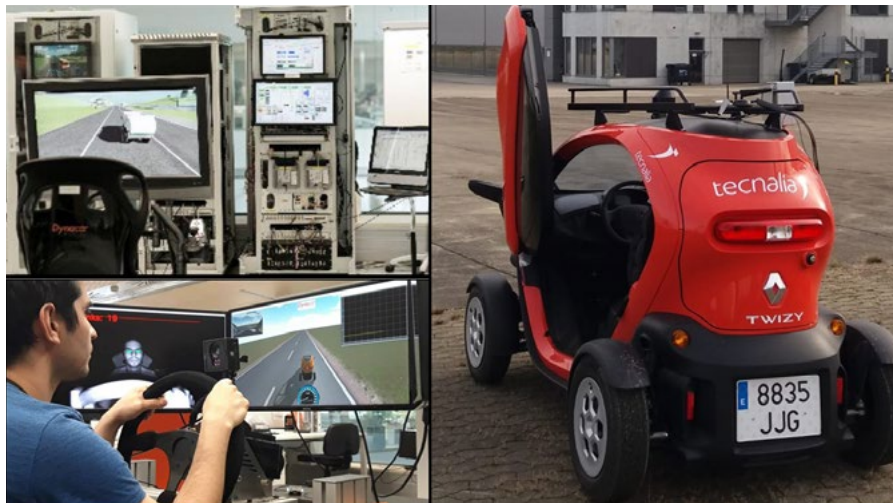
Advanced control system laboratory, shared control simulator and connected and automated Twizy vehicle
