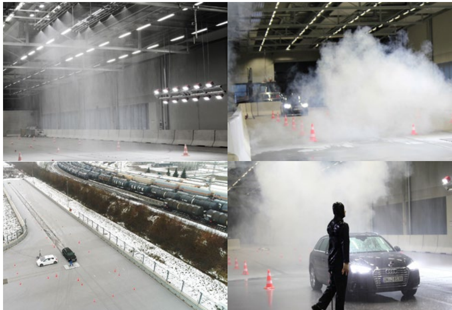
Outdoor and Indoor CARISSMA Test Facilities under weather conditions (Rain and Fog Simulation Tests)
