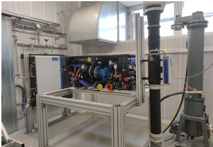
Fuel cell test bench, designed for 200 kW FC and with capabilities for hardware-in-the-loop developments
