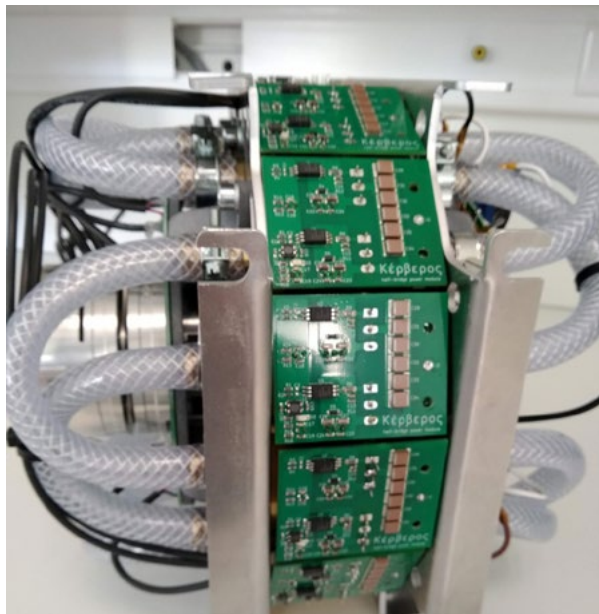
Axial flux electric machine with integrated power electronics
