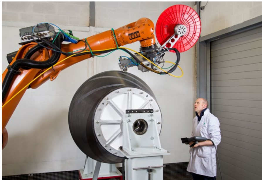
Laser-assisted tape placement (LATP) of carbon-fibre based thermoplastic composites using the LATP in the Irish Composites Centre (IComp), University of Limerick.
